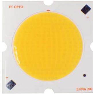
**Luna 200** Chip on Board is a high-performance LED module based on patented **DBR Flip Chips** and unique low temperature bonding technology. The magnitude of the LED illumination is enhanced by the DBR structure to further increase the lighting efficacy. Additionally, the embedment between LED flip chips and MCPCB as well lowers the thermal resistance.
